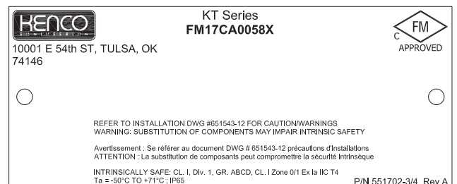
Figure 21: Intrinsically Safe Digital Output Label (Canada)
